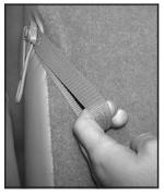
Pull up on the release lever labeled 1 and then pull up on the seatback or the assist strap located on the outboard side of the seat until the seatback locks into the upright position.
